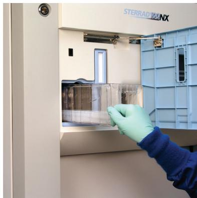
**Figure 74. Open the Access Panel and Remove the Used Cassette Disposal Box by Pulling on the Tab and Sliding the Box Out.**
