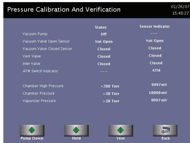
**Figure 91. Pressure Calibration and Verification.**
