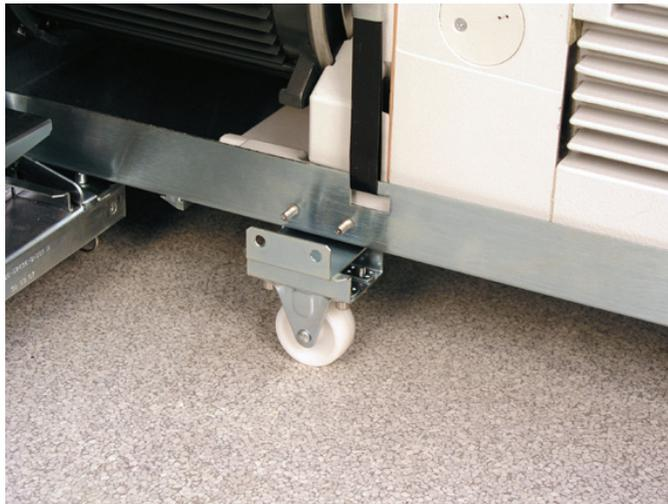
*Note: The castor assembly can only fit one way on the tray. Ensure proper orientation.*
