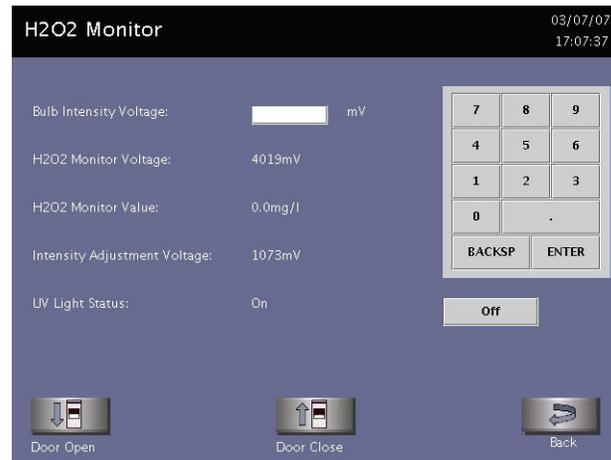
**Figure 98. H<sub>2</sub>O<sub>2</sub> Monitor.**
