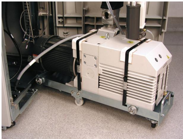
**Figure 67. Vacuum Pump Assembly Shown Removed from the System.**
