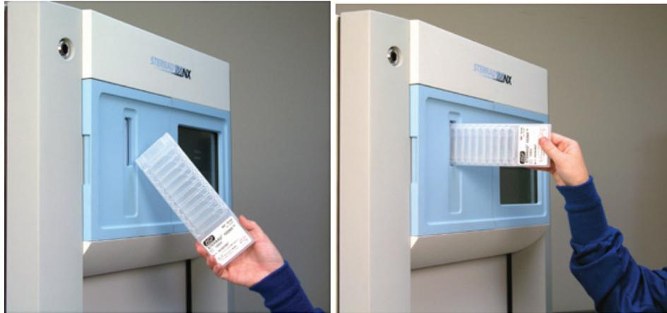
**Figure 37. Inserting the Cassette into the Slot.**
