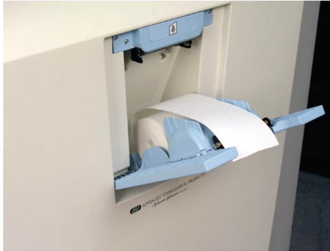
**Figure 78. Insert a New Paper Roll. Pull the Paper Over the Top of the Door and Align the Paper Between the Guides.**
