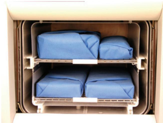
**Figure 35. Load Correctly Placed.**
