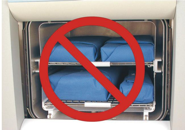
**Figure 33. The Load Should NOT Touch the Electrode.**
