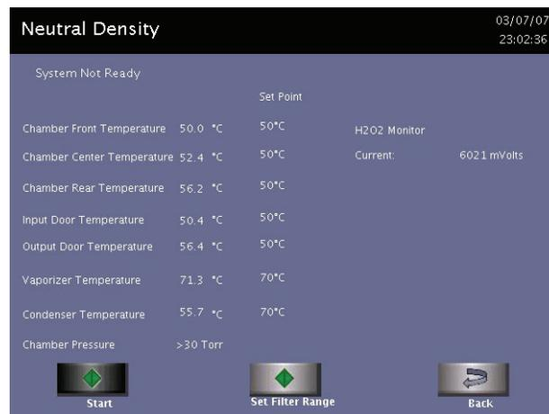
Figure 86. Neutral Density Filter Calibration Display. Note that Start is Inactive.
