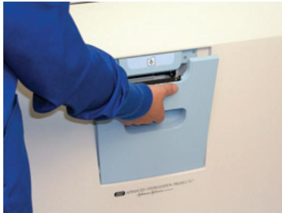
**Figure 76. Open the Printer.**
