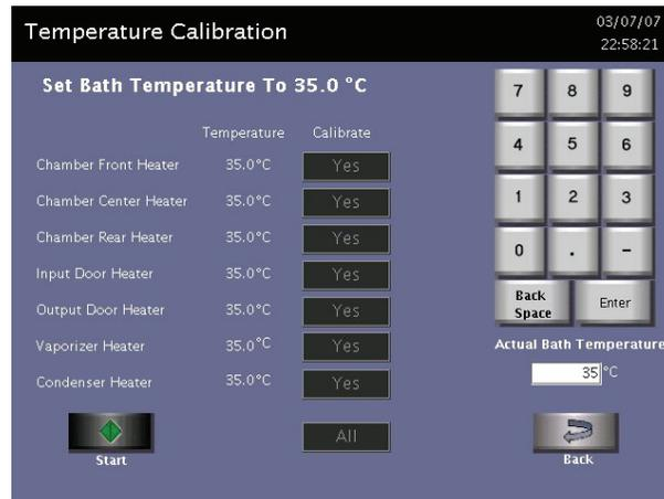
**Figure 81. Temperature Calibration Showing Virtual Keypad.**
